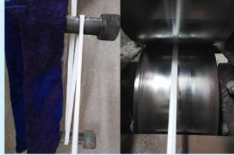
4. Stretching and roll forming
